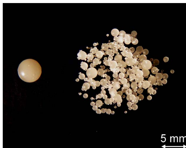
Fig. 1. Silicone spheres with lipase-containing static emulsion. Bead diameter was up to 4 mm, depending on the stirring intensity of the PVA-hardening bath during preparation.
